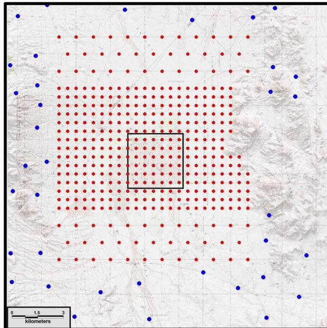
**FIGURE 9: Proposed Gravity Stations over Topography**
