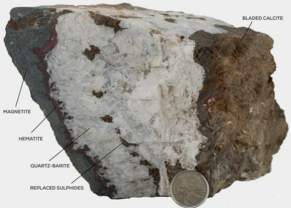
Above: Barite-Quartz-Magnetite vein with hematized wall rock, boiling textures and oxidized sulphides within the vein. This sample was hosted in Nicol Creek Basalts.
