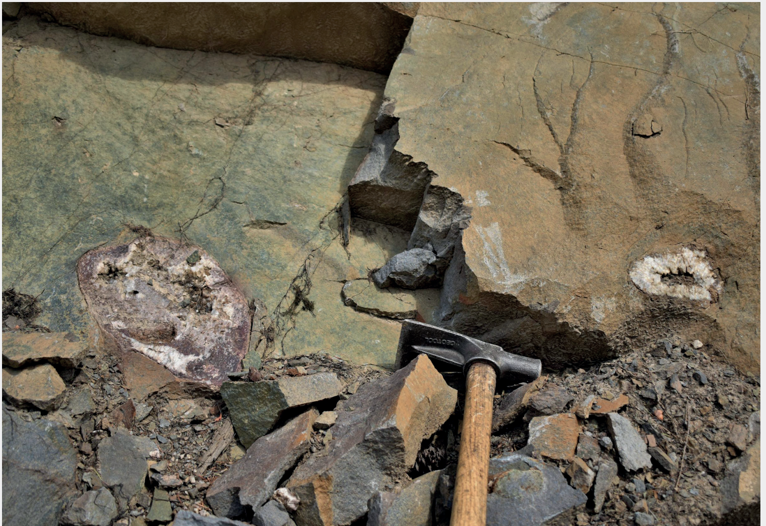
Below: Geodes within Nicol Creek Basalt – open voids, well developed quartz and barite crystals with hematized/magnetite-altered wallrock.
