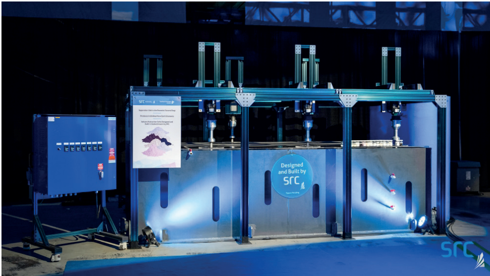
Grand Opening: Canada's first proprietary solvent extraction cell technology for REE processing was presented by the Saskatchewan Research Council (SRC) in May 2023.
