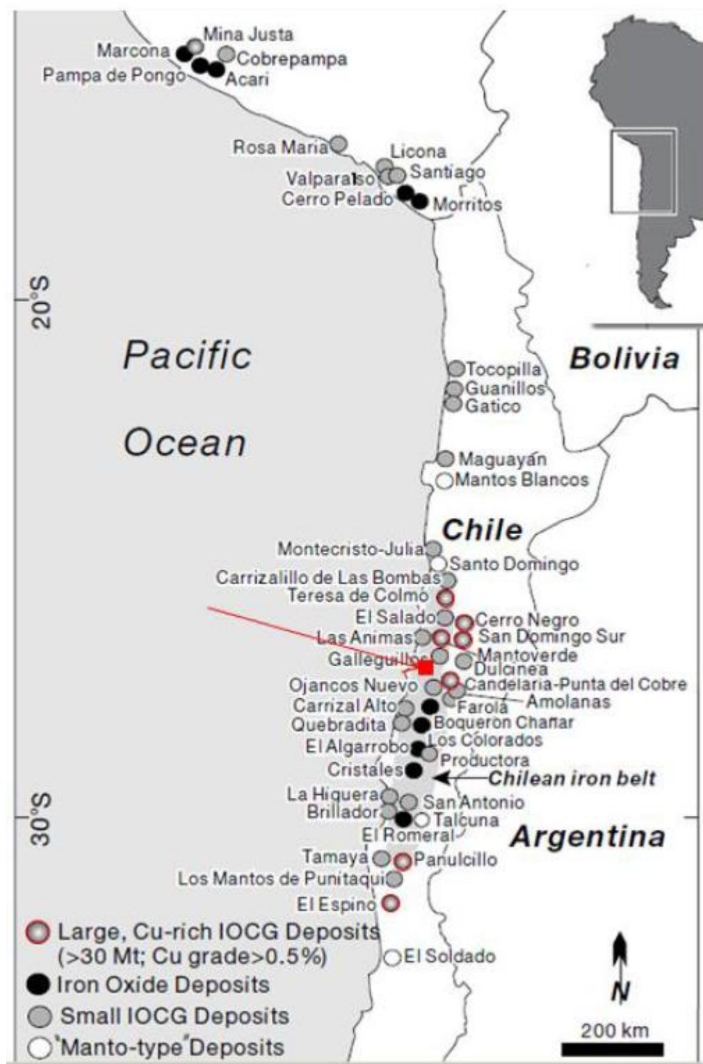
Figure 8-1: Map of southern Peru and northern Chile showing the location of Iron Oxide (-Apatite - IOA) and Iron Oxide-Copper-Gold (IOCG) deposits. Note the overlapping relationship between Magnetite-apatite (IOA) deposits and Iron Oxide-copper-gold (IOCG) deposits). (Mining Group 2013c).
