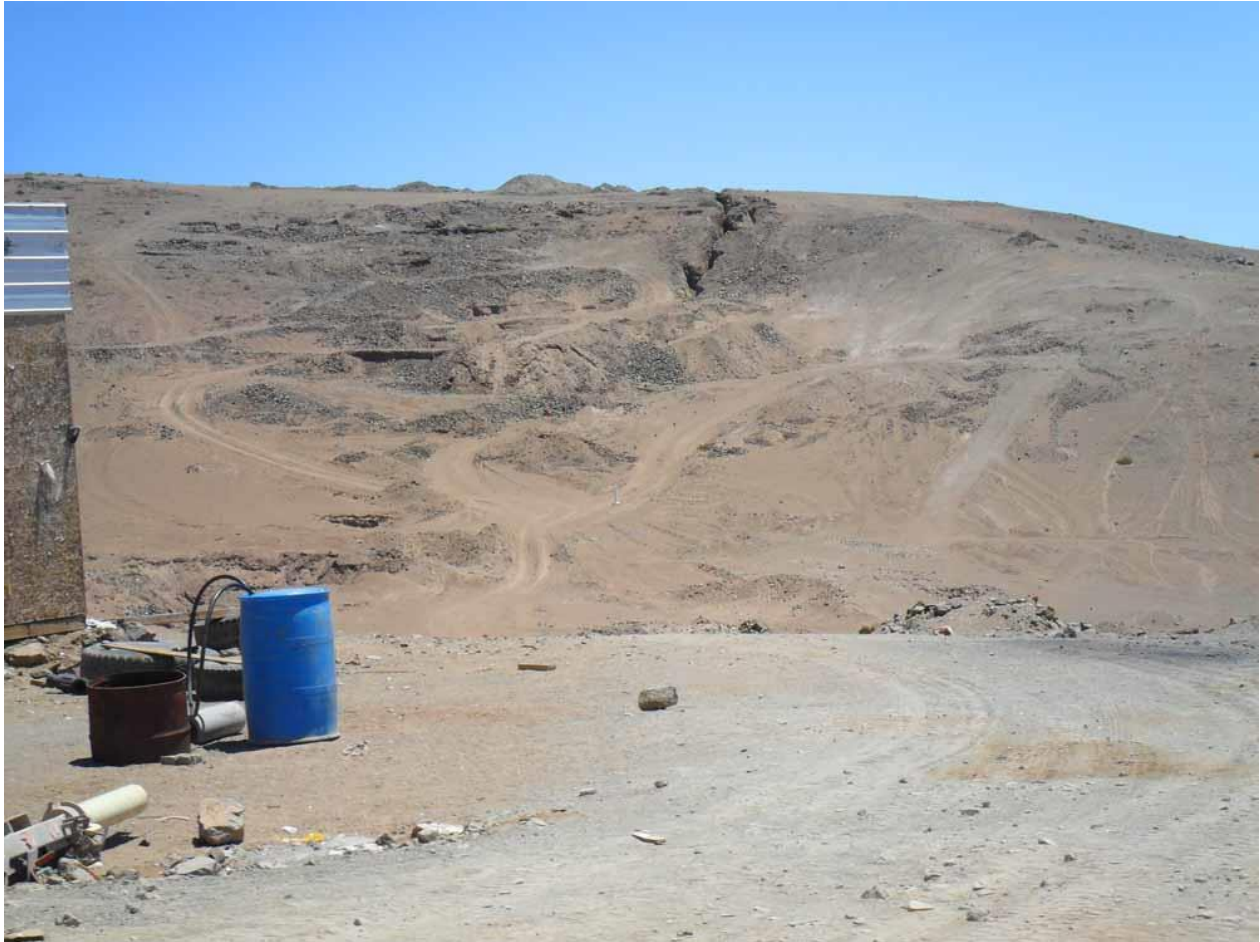
Figure 6-11: Aguilander workings developed along next major vein, Major Vein #2, to the north of Descubridora. Numerous, smaller workings have been developed along veins, presumably smaller and/or discontinuous, between the major veins. In addition, numerous “waste” piles from current and historical workings are abundant in association with all workings. View to west-southwest. Photo by R. Walker, 2012
