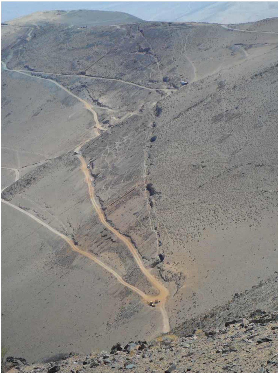
Figure 6-10: Detail of the workings developed along Major Vein #1 (Descubridora), with Caupolicán in foreground (east) and Rincon (on skyline), with Viuda and Estaca located farther west. View west-southwest from peak at 346354 E, 7008678 N (WGS 84). Photo by R. Walker, 2012
