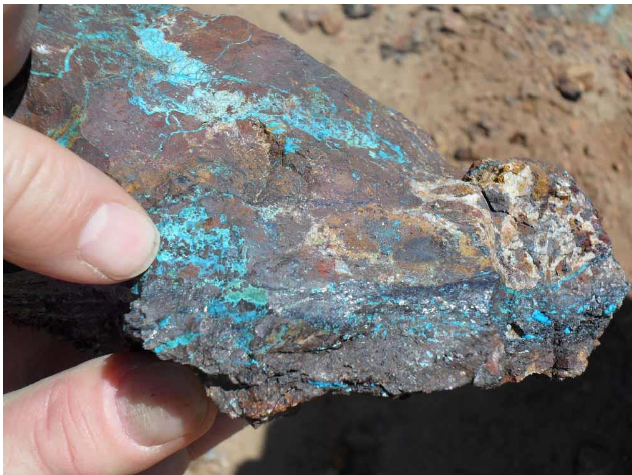
Figure 6-14: Close-up of high-grade mineralized material comprised of dark reddish brown “almagradito”, with development of secondary azurite (blue) and subordinate malachite (green). Minor development of dark brown limonite to goethite, annealed by local stockwork of calcite veins at right edge of photo. Possible vein of high grade, black chalcocite developed parallel to lower margin of sample, just below finger. Photo by R. Walker, 2012
