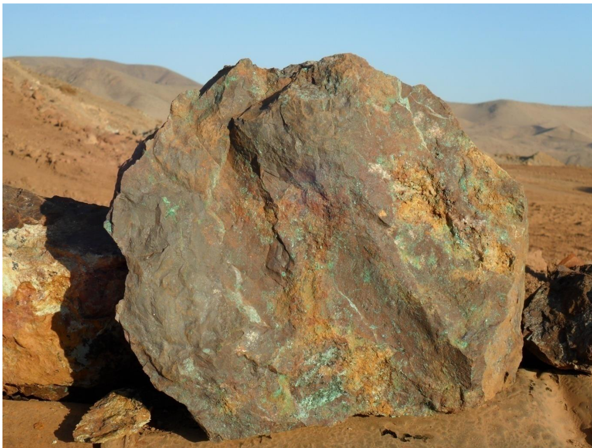
Figure 8-6: Example of “almagadro”, an intimate mix of high-grade copper minerals and hematite. This sample is from the Veta Gruesa Centre drift and representative of Direct Shipping Mineralized Material, grading approximately 9% copper (Cu). Photo by R. Walker 2012.
